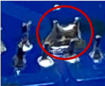
Small solder bridge that needs to be removed.
