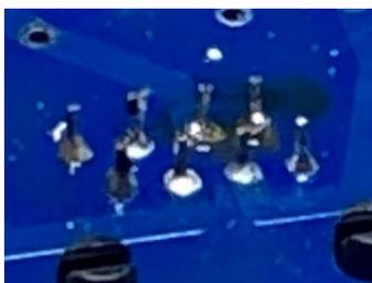
Terminals after removing the solder bridge.
