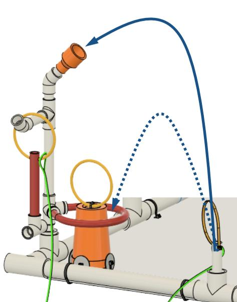
Temperature Sensor Connector Placement
